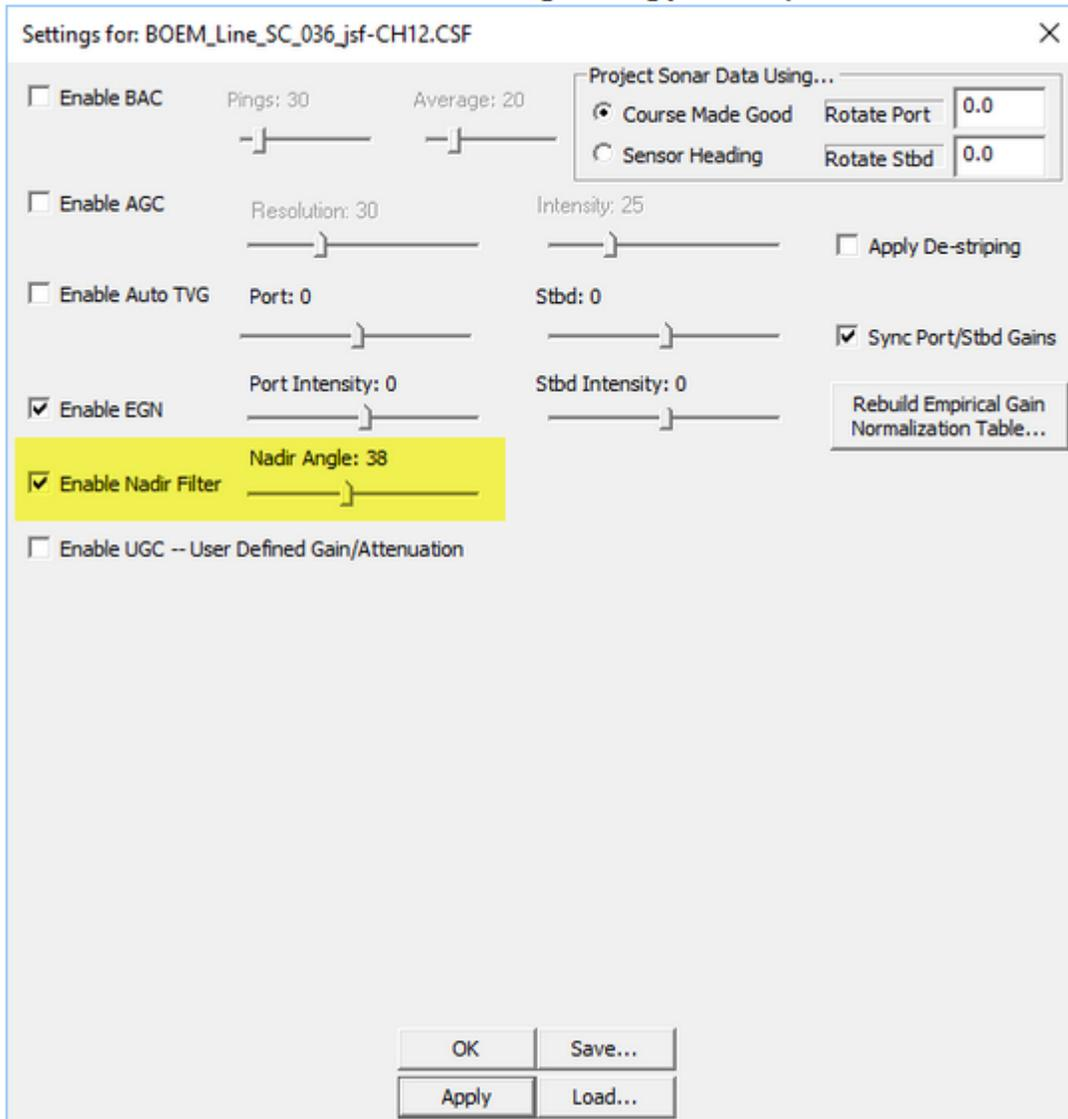
The angle setting is the aperture angle from the sonar straight down under the towfish that will be filtered. So, larger angles affect a wider nadir swath.
