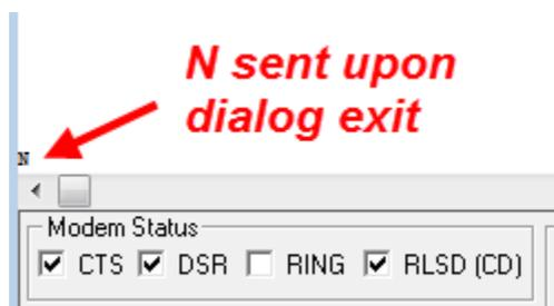
This N is seen in the MTTY.exe application, where we have used VSPE to record from COM2, and SonarWiz is connected to COM3, and VSPE (Eterlogic.com, virtual serial ports emulator) creates the COM2=COM3 pairing.
