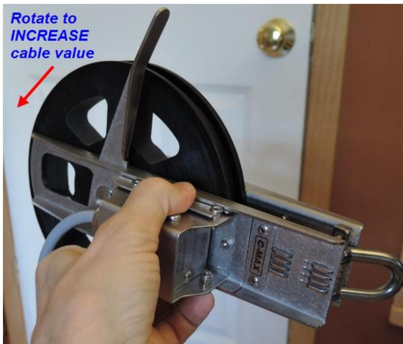
and the meters cable-out number increased from 15.0 to 16.0:
