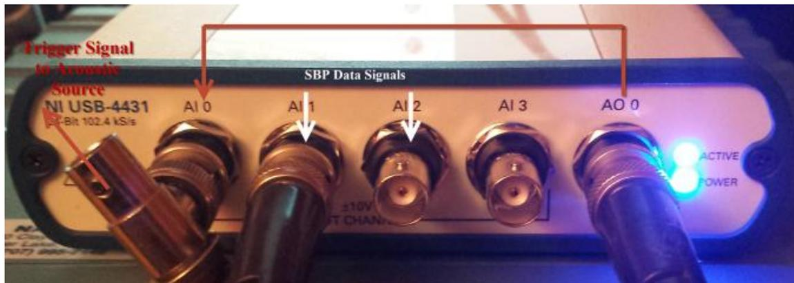
**Nota bene:** Please be sure to test trigger use with your actual equipment before a survey, as it may not be a TTL-compatible voltage range, though it is a square-wave signal output. If you will need an intermediate pre-amp stage to make this perfectly TTL-compatible, better to find this out in a lab test, before discovery at the boat.
