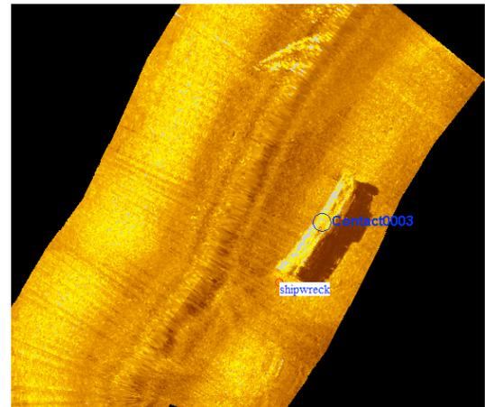
*Sample output generated by SyQwest AquaScan and SonarWiz 5 showing a shipwreck.*
